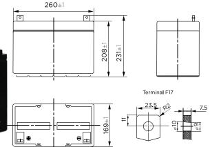
These rechargeable batteries are lead-lead dioxide systems. The dilute sulfuric acid electrolyte is absorbed by separators and thus immobilized. Should the battery be accidentally overcharged producing hydrogen and oxygen, special one-way valves allow the gases to escape thus avoiding excessive pressure build-up. Otherwise, the battery is completely sealed and is, therefore, maintenance-free, leak proof and usable in any position.
