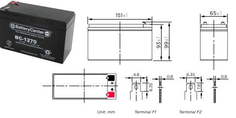
These rechargeable batteries are lead-lead dioxide systems. The dilute sulfuric acid electrolyte is absorbed by separators and thus immobilized. Should the battery be accidentally overcharged producing hydrogen and oxygen, special one-way valves allow the gases to escape thus avoiding excessive pressure build-up. Otherwise, the battery is completely sealed and is, therefore, maintenance-free, leak proof and usable in any position.
