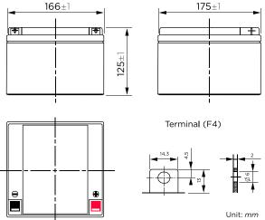
These rechargeable batteries are lead-lead dioxide systems. The dilute sulfuric acid electrolyte is absorbed by separators and thus immobilized. Should the battery be accidentally overcharged producing hydrogen and oxygen, special one-way valves allow the gases to escape thus avoiding excessive pressure build-up. Otherwise, the battery is completely sealed and is, therefore, maintenance-free, leak proof and usable in any position.
